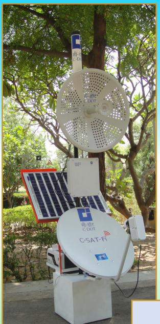
C-DOT Satellite Wi-Fi (C-Sat-fi) is an innovative integration of VSAT Technology with C-DOT BBWT\* Wi-Fi Terminals. The satellite connectivity is used as Backhaul link for the complete village. C-DOT BBWT Wi-Fi such as Solar Wi-Fi is used for Hotspot and C-DOT Long Range Wi-Fi is used as Point to Point & Point to Multi Point links to cover the complete village.
